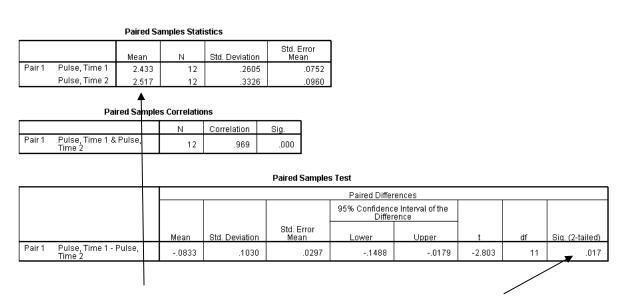
By looking at the sample means one can see they are different. The p value is 0.017 showing that the t value is significant.
