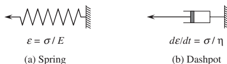
Figure 5-52 Spring and dashpot for modeling viscoelastic behavior
