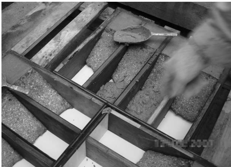
Figure 6-38 Casting of prisms for slant shear measurement
