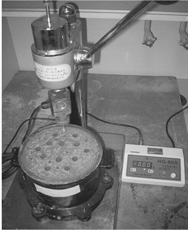
Figure 3-8 Measurement setup of concrete mixture setting time
