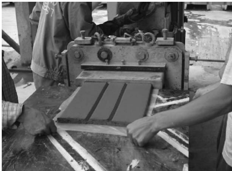
Figure 6-6 The extrusion process
